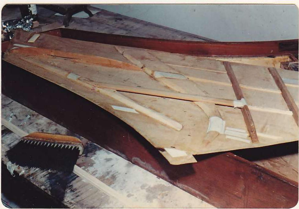
Detail of Unusual Soundboard barring
